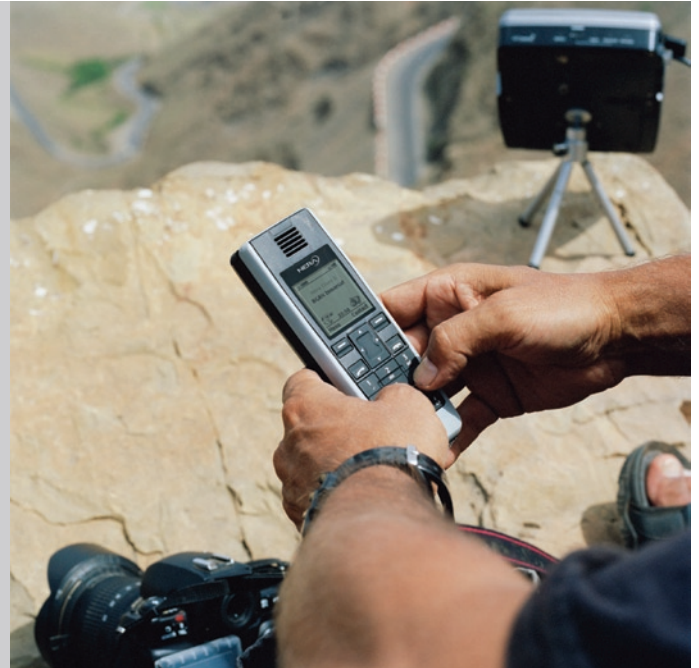
Configuring and controlling the Nera WorldPro 1000 directly from the handset.
